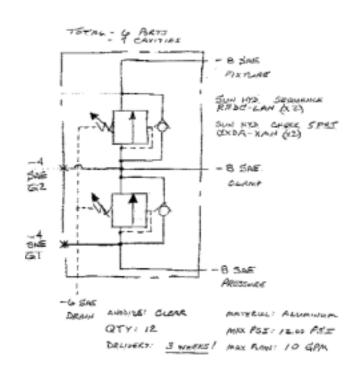
Your specs can be simple or complex, tight or rough. We'll turn them into finished integrated hydraulic circuits.
