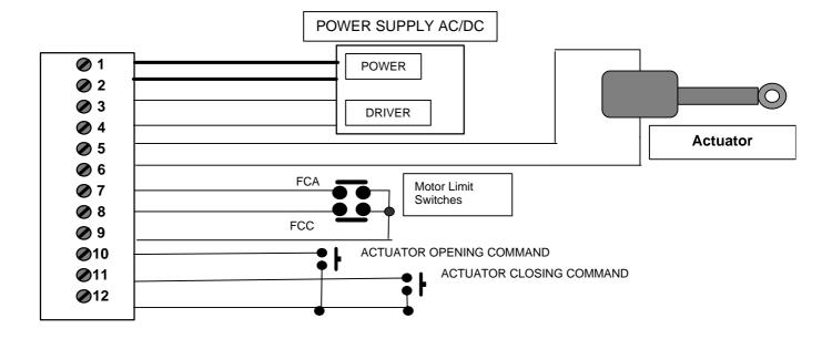
FCA = OPEN POSITION Limit switch FCC = CLOSE POSITION Limit switch
