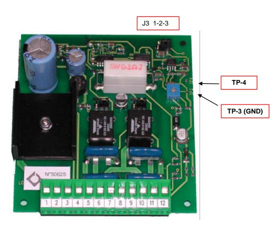
J1-J2Actuator Limit switches jumpersJ3Actuator Current Limitation jumperP1Trimmer for Actuator current limitation adjustment
