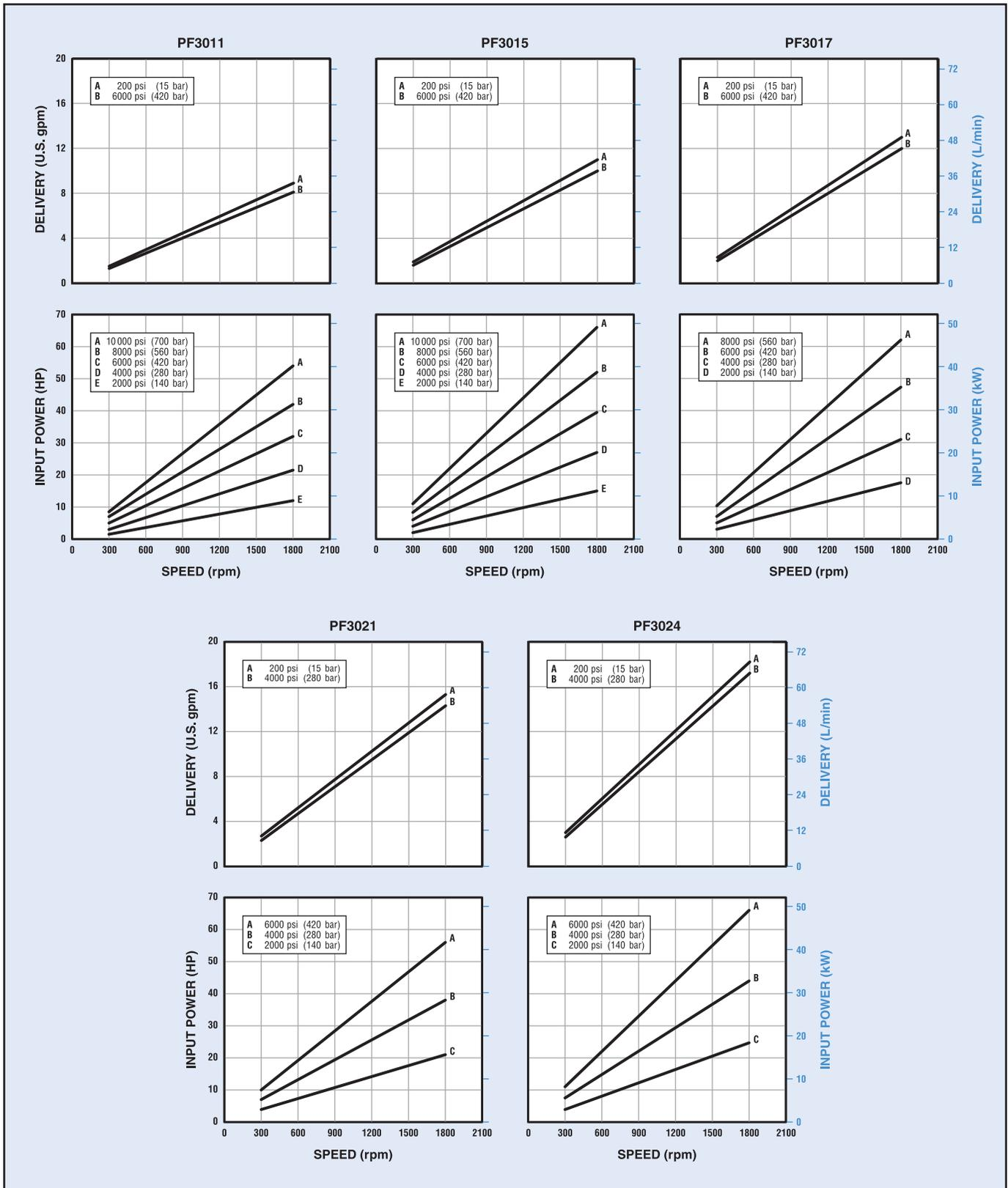
Typical performance curves are based on 100 SUS (20 cSt) mineral oil with pressurized inlet where required. Refer to "Minimum Inlet Pressure" table on page 2.
