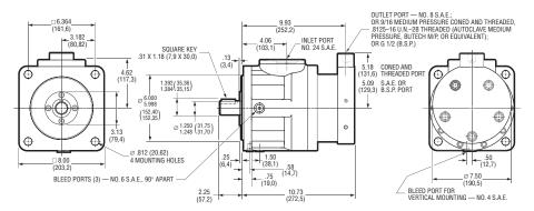
Dimensions are shown in inches (millimeters in parentheses) and are nominal. The drawing shows a standard keyed shaft. Contact the sales department for port and shaft options, and for complete installation and operating recommendations.
