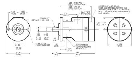
Dimensions are shown in inches (millimeters in parentheses) and are nominal. The drawing shows a standard keyed shaft. Contact the sales department for shaft, port and seal options, and for complete installation and operating recommendations.
