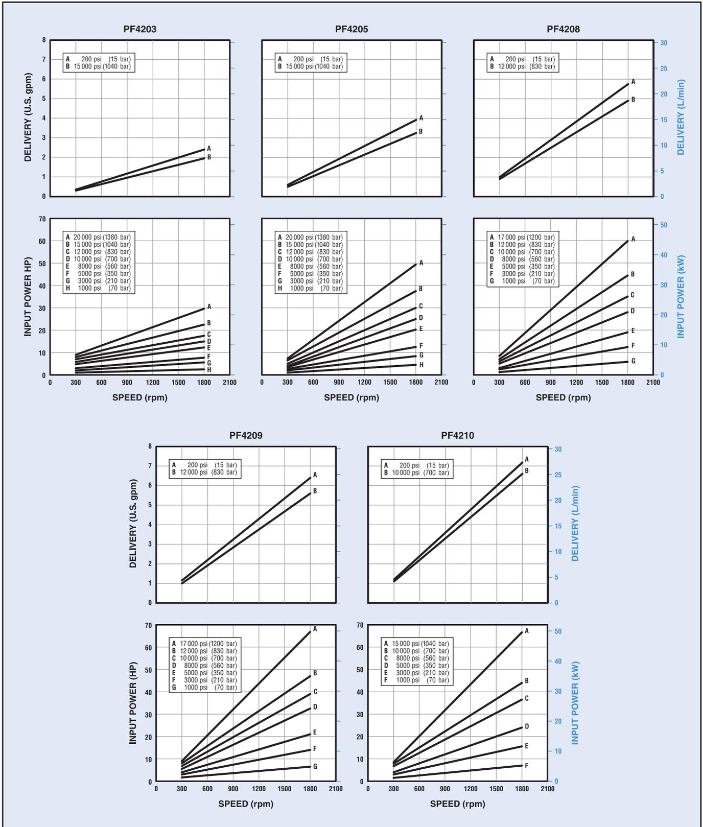
Typical performance curves are based on 100 SUS (20 cSt) mineral oil with pressurized inlet where required. Refer to the "Minimum Inlet Pressure" table on page 2.
