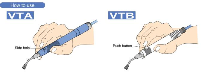
Send compressed air of 0.5MPa(72.5psi) to the air pincette. Close the side hole (the push button) with your finger to hold the work under suction. And open the side hole (the push button) to release the work.
